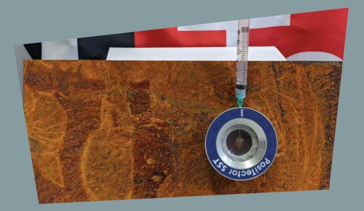
THE AVERAGE READINGS WERE AS FOLLOWS: **TOTAL SALT:** 115.7  $\mu$ g/cm<sup>2</sup> **TOTAL CHLORIDES:** 36  $\mu$ g/cm<sup>2</sup>
