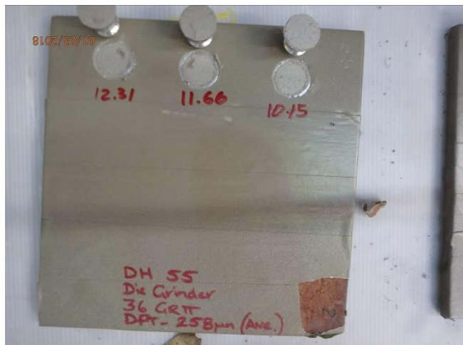
Figure 8- DH55 Pull off test on #36 grit grinder wheel
