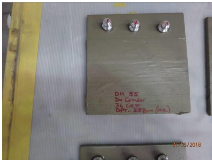
Figure 7- Pull off Dollies were glued several days before the 1.3.2018
