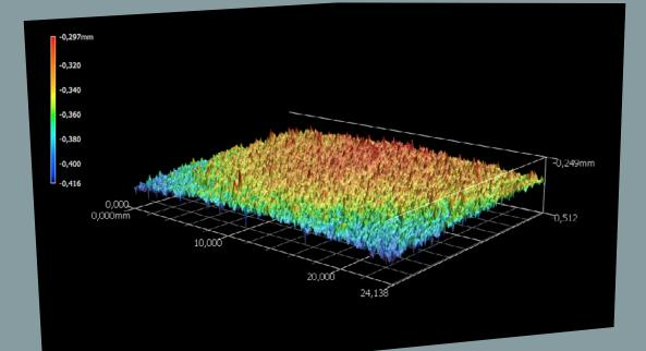
More peak counts and peak density provides a steeper profile. At the other hand, a too high peak counts and peak density will have a negative affect on coating performance, because there is a risk not wetting the substrate completely with coating. This creates voids on the substrate/coating system interface, which is not desirable for multiple reasons.
