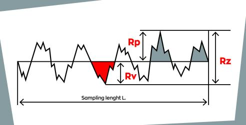
**RP** = the largest profile peak height and **RV** the maximum profile valley depth within one of the five sampling lengths of the measurement length I.
