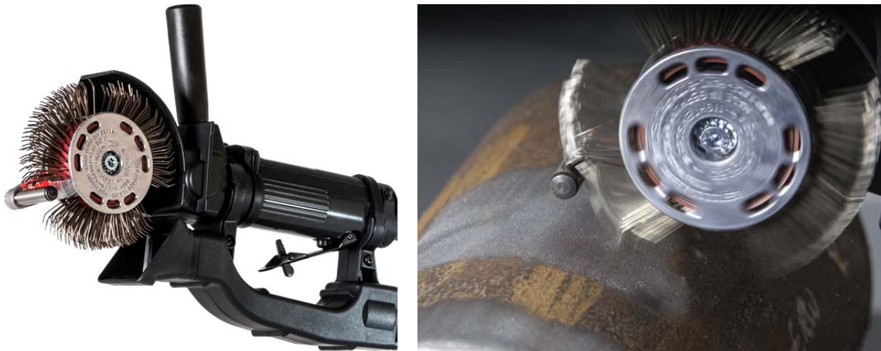
Figure 3: Bristle Blaster® tool for wire bristle impacting
